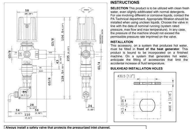
Choose a correct nozzle size, which allows a regular discharge on bypass, at least 5% of the total flow of the system in order to achieve a constant pressure value and avoid troublesome pressure spikes at closure. If the nozzle wears out, the pressure drops. On installation of a new nozzle, re-adjust the system to the original pressure setting. Electrical installation must be carried out by qualified personnel
